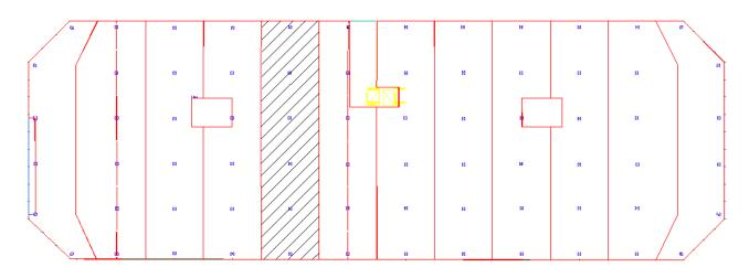
Figure 10: Post-Tension design Strips in N-S Direction (Residential floor)
