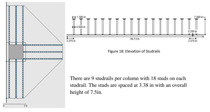
Figure 19: Plan of Studrails
